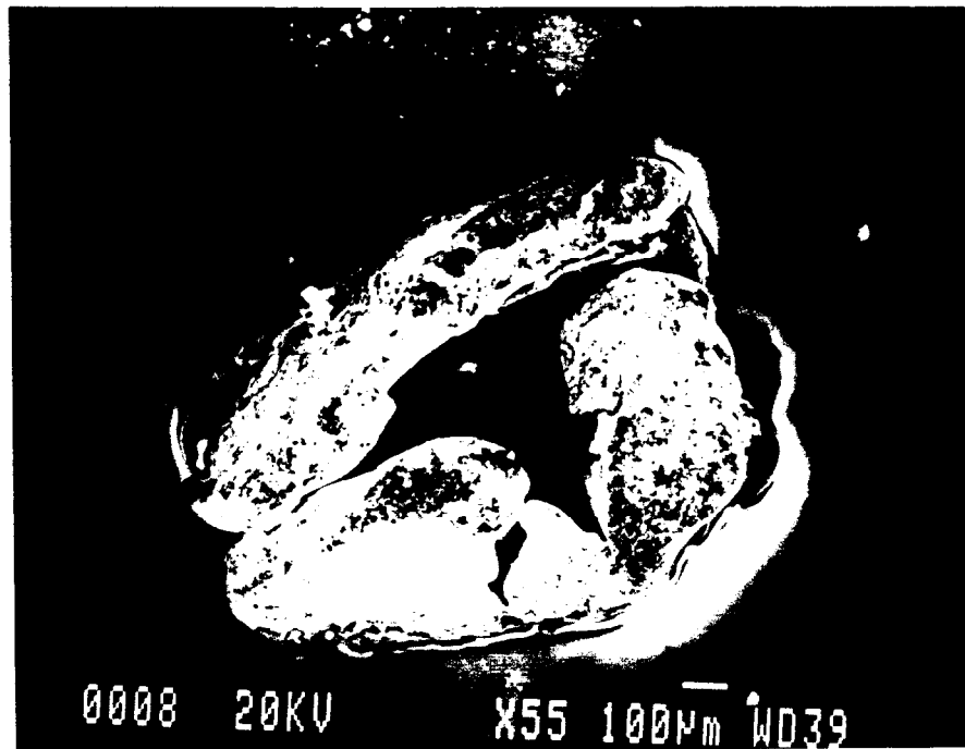
Figure 9 Initial Stage of the Folding of a Gold Flake in a Spherical Shape
