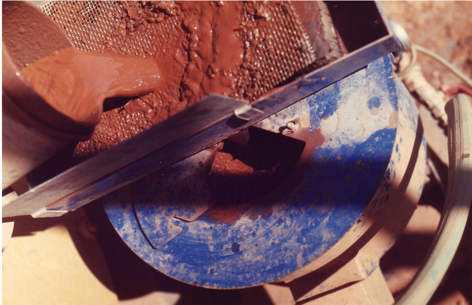
A close up of the feed coming from the ball mill to 7.5" concentrator.
