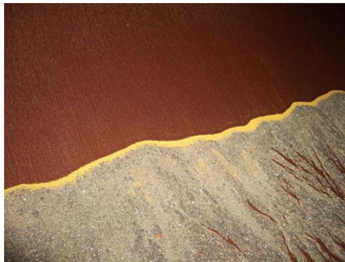
Figure 1 High-grade gravity concentrate produced by Knelson Concentrator at Gorubso-Kardjali
