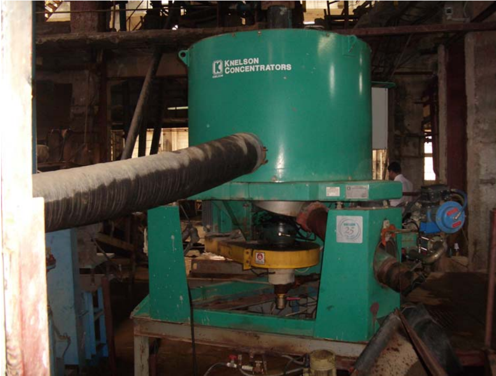
Figure 2 Knelson KC-CD30 at Gorubso-Kardjali processing facility in Bulgaria
