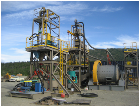
Prize Mining Gravity Plant Supplied by Knelson Gravity Solutions
