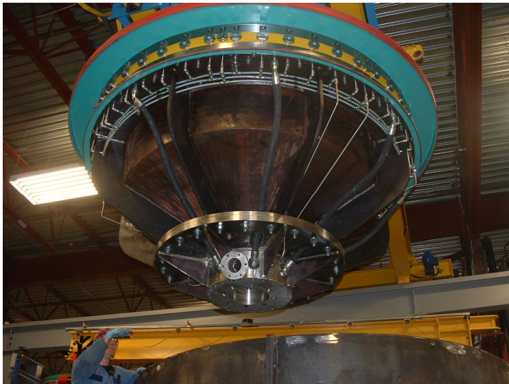
CVD64 Rotor Assembly is lowered into position
